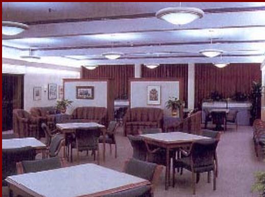
Figure 1 Pendant + Cove Lighting
